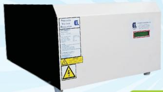
ETIPL's automatic precision line voltage Conditioner provides output voltage within ±2% of nominal, for input voltage that varies between 175-280 VAC\*.PVr is compatible with all loads as it does not switch any components in the power path. There is no electrical motor used for slow correction of output voltage and possibility of over-voltage by system itself.
